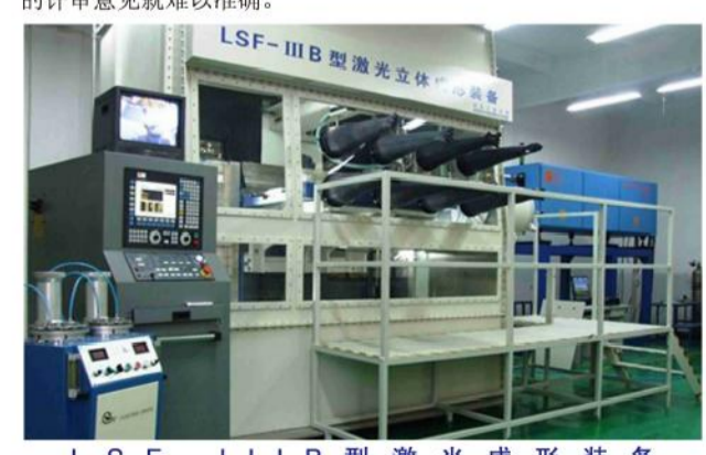
LSF-III B型激光成形装备
